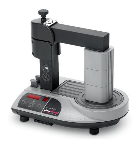
The medium-sized simatherm induction heater for roller bearings and other circular metal workpieces up to 400 mm bore diameter and a cross section of 145 x 205 mm. With the integrated time and temperature controls, roller bearings can be heated to the prescribed 110°C while other circular metal workpieces can be heated to 400°C.
