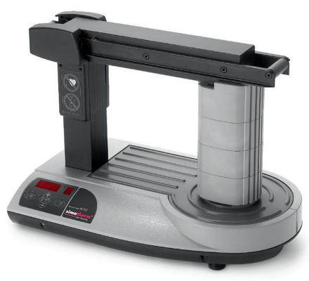
The large simatherm induction heater for roller bearings and other circular metal workpieces up to 640 mm bore diameter and a cross section of 250 x 250 mm. With the integrated time and temperature controls, roller bearings can be heated to the prescribed 110°C while other circular metal workpieces can be heated to 400°C.
