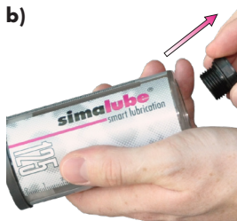
b) Remove gas generator with a socket wrench (SW21 mm)
