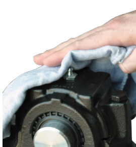
Clean lubrication point
