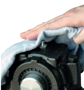
Clean lubrication point
