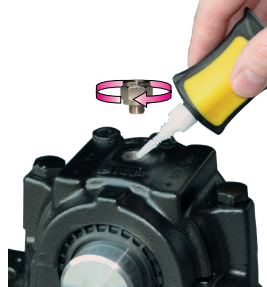
Screw in reducing nipple (if necessary, seal lubrication point)
