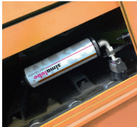
The conveyor belt chain in a recycling factory is automatically lubricated and cleaned with simalube and brush.
