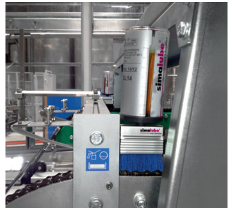
simalube and brush lubricate the chain in a brewery.
