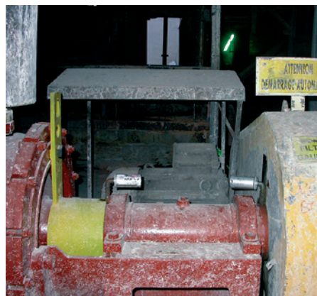
Permanent bearing lubrication on the main drive shaft of a filter pump.
