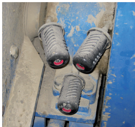
Protective caps used to prevent damage to the lubricator from harsh external conditions.
