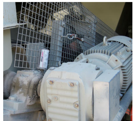
A vertical bearing on a conveyor belt is lubricated with a simalube lubricator.
