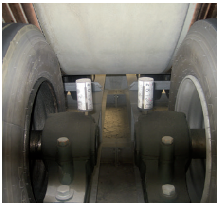
The lubricators are connected directly to the vertical bearing on the drive of a conveyor belt.
