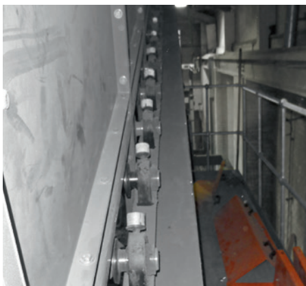
Dozens of 30 ml simalube lubricators provide the bearings of a conveyor belt with the necessary lubricant.
