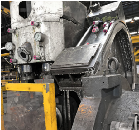
Several simalube lubricators and IMPULSE lubricate the columns (left) and the drive unit (right) of the nibbling machine.
