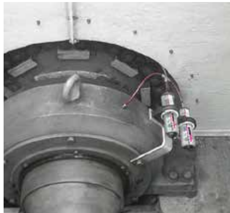
Two simalube 250ml lubricators lubricate the main bearing of a wind turbine.
