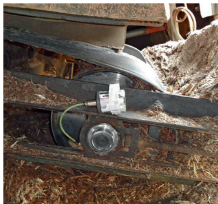
The Y-ball-bearing unit of a conveyor belt is continuously supplied with lubricant.
