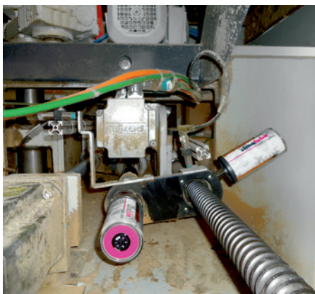
The spindle of a circular saw is reliably lubricated with two 125 ml simalube cartridges.
