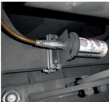
The 125 ml dispenser is installed on the chassis of a low floor tram. The lubricant is directed through a hose to the lubrication point.
