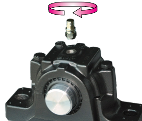
Remove connector nipple and screw in quick connection coupling
