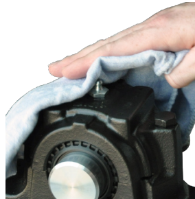
Clean lubrication point
