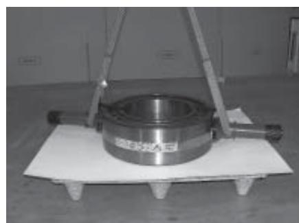
The length of the slings (L) must correspond the bearing diameter (D) to 1.5.
