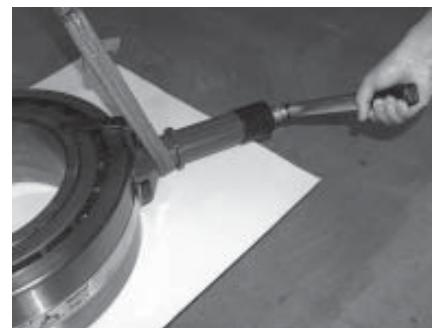
For some types of bearing, the inner ring must be locked to prevent rotation of the inner ring. This does apply for spherical roller bearings. Loosen the inner ring holders and place them against the bearing inner ring. When in the correct position, retighten the inner ring holders.
