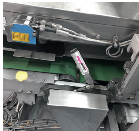
Bearing lubrication of the drive roller of a conveyor belt in the production of chips (crisps).
