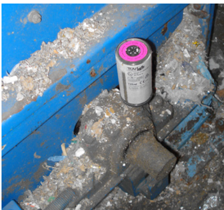
In a paper factory the pedestal bearings of a shredder are lubricated with a 125 ml simalube unit.
